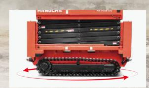
The steering proportional deceleration and electronic differential function can make the machine pivot steering.
